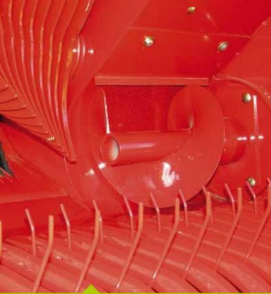
**Cross feed in the pick-up via counter-rotating spirals**This achieves an effective and secure bale material compaction, even on wide swaths. The bale chamber is thereby optimally filled and the cutting quality is superb.
