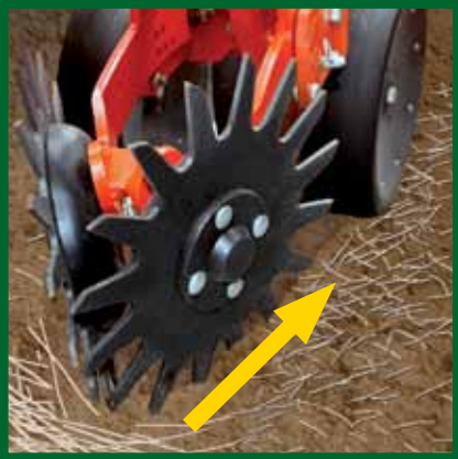
Trash Wheels The adjustable trash wheels clean the row sweeping crop residues away. They prevent from uneven gauge wheels depth control and from trash burying.
