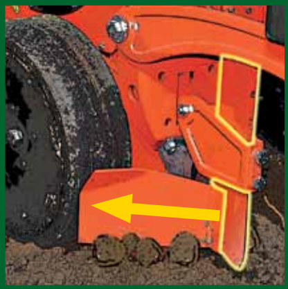
Clods Pusher The adjustable clod pusher moves dry soil and clods away from sowing slot, the front mounted independent coulters can cut the soil for a prime furrow opening on tilled soils conditions.
