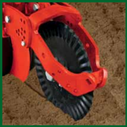
Front disc Unit front mounted disc coulters cuts into hard soil in reduced till conditions. The wave profile creates extremely fine tilth 7/8 wide slot. Suitable for wet, spongy soils where it can be difficult to close the furrow.
